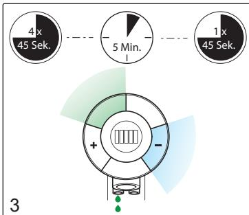
Activate the soap and “-” sectors at the same time. After 45 seconds the pump will automatically stop. Repeat this 4 times.
