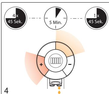
Remove the TubeCleanse solution from the left side of the Soapbox and install it on the right side of the Soapbox. Activate the disinfectant and “+” sectors at the same time. After 45 seconds the pump will automatically stop. Repeat this 4 times.
