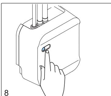
Press the blue LED button to exit priming mode.
