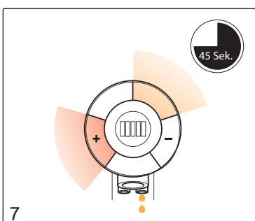
Activate disinfectant and “+” sectors to prime disinfectant tube. After 45 seconds the pump will automatically stop.
