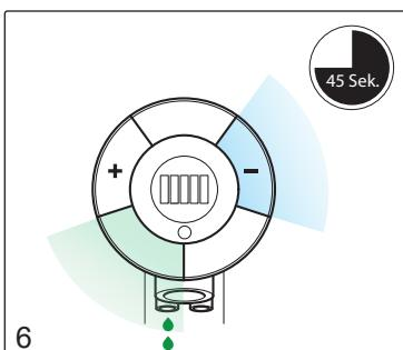
Activate bottom left sector and “-” sector to prime the soap tube. After 45 seconds the pump will automatically stop.
