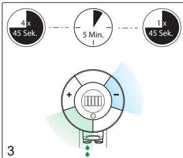
Activate the left bottom sector and “-” sector at the same time. After 45 seconds the pump will automatically stop. Repeat this 4 times.
