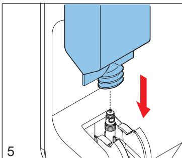
Remove the TubeCleanse solution from the soapbox and install new liquids into the soapbox.
