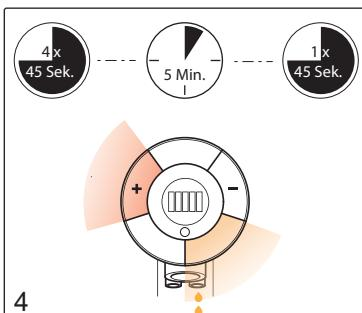
Remove the TubeCleanse solution from the left side of the Soapbox and install it on the right side of the Soapbox. Activate the bottom right sector and “+” sector at the same time. After 45 seconds the pump will automatically stop. Repeat this 4 times.
