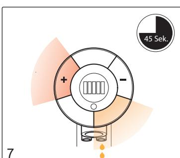
Activate bottom right sector and “+” sector to prime remaining tube. After 45 seconds the pump will automatically stop.
