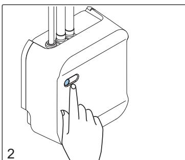
Press the blue LED button on the waterbox to activate priming mode. The blue LED light will start blinking.
