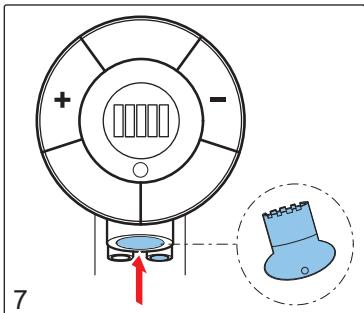
Use the perlator key to install the new aerator provided in the SystemCare Set.
