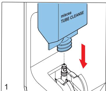
Install the two pouches of TubeCleanse solution on the Soapbox.
