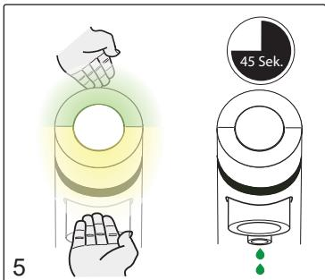
Activate soap sector and water sector to prime the soap tube. After 45 seconds the pump will automatically stop.
