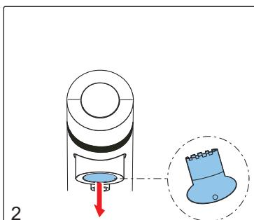
Remove the aerator from the water outlet with the perlator key provided.
