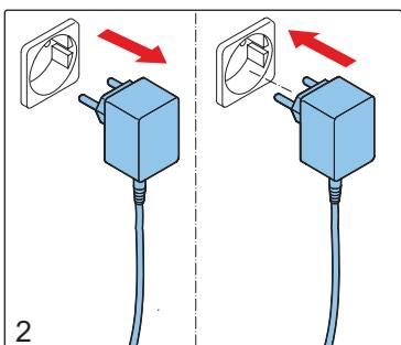
Enter the priming mode by first unplugging the power adapter, and then plugging it back in again.
