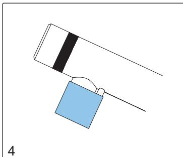
To decalcify the water outlet, fill the round plastic container provided with water and vinegar to a ratio of 1:1. Then carefully submerge the water outlet and dispenser outlets into the water and vinegar solution.
