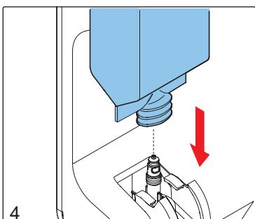
Remove the TubeCleanse solution from soapbox and install new liquids into soapbox.
